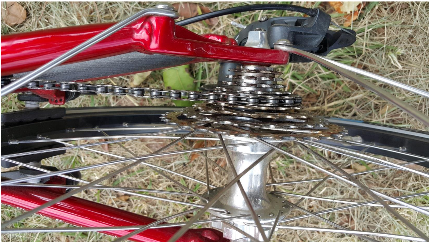
Nine sprockets on the rear and three on the front make it a 27 speed.
