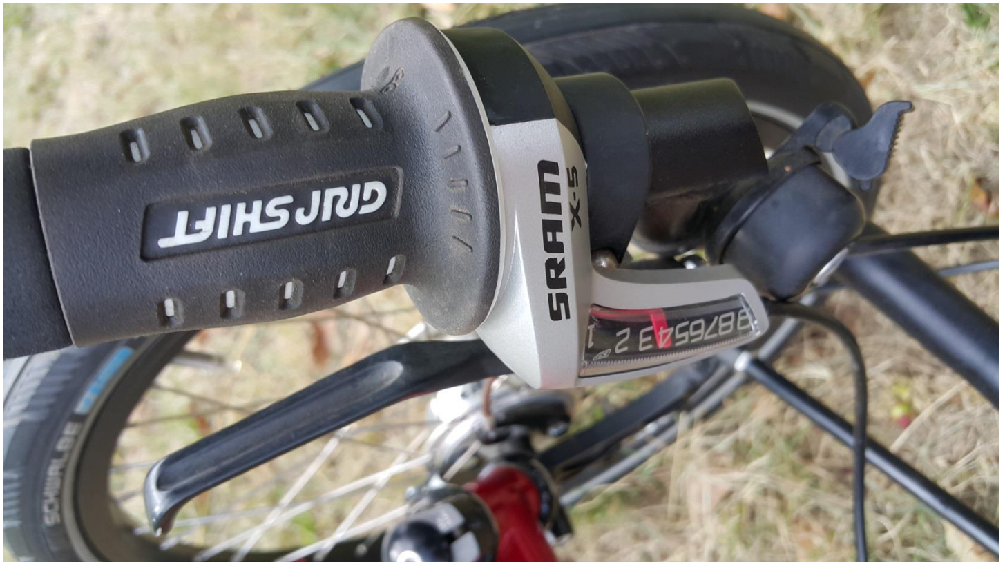
The shifter to adjust the nine sprockets at the rear wheel.
