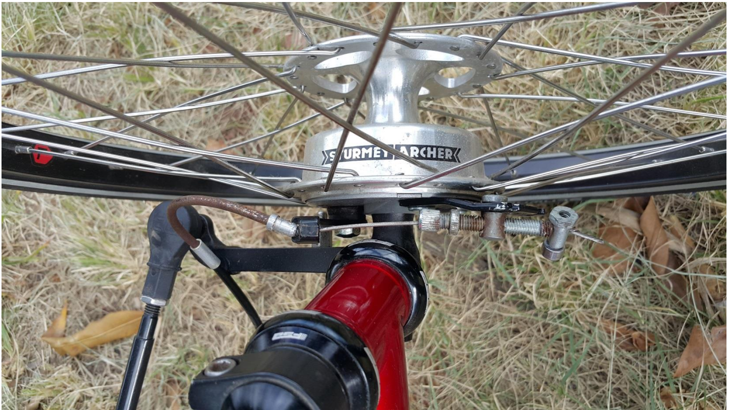
A good drum brake system on each of the front wheels.
