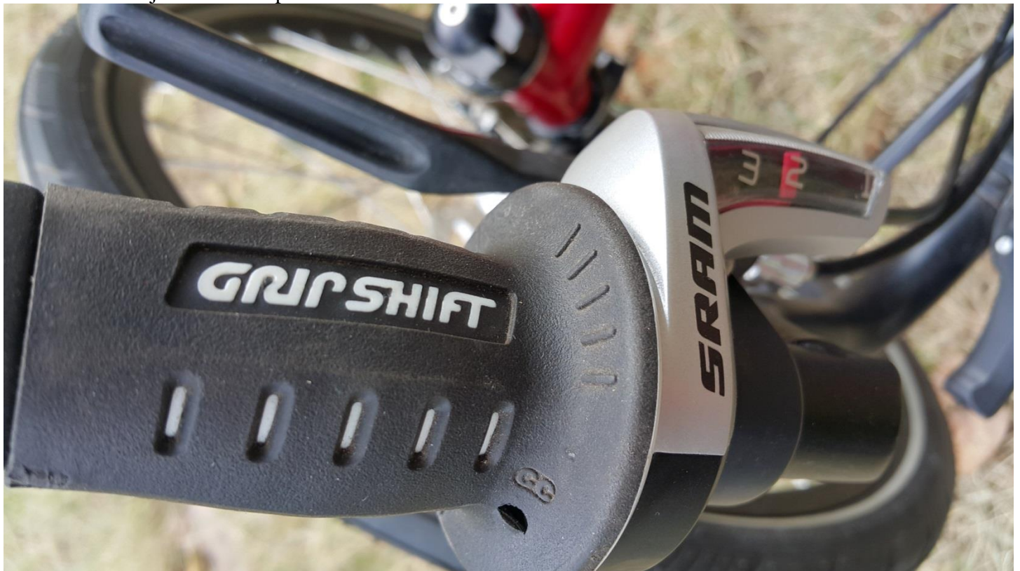
This shifter adjusts the three sprockets at the front.
