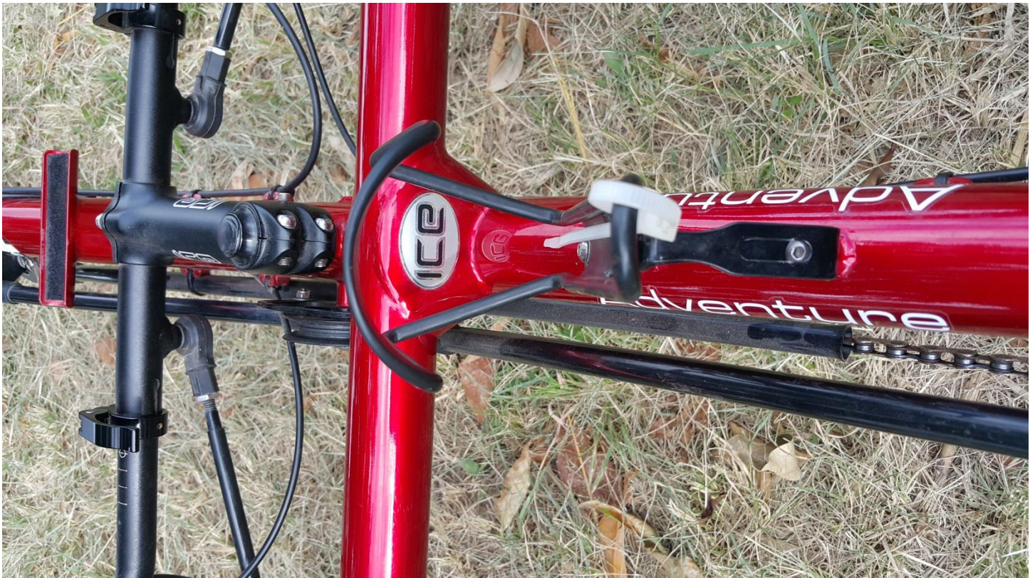
The handle bars, used for steering, are adjustable in and out for width and tilting forward or backward.
