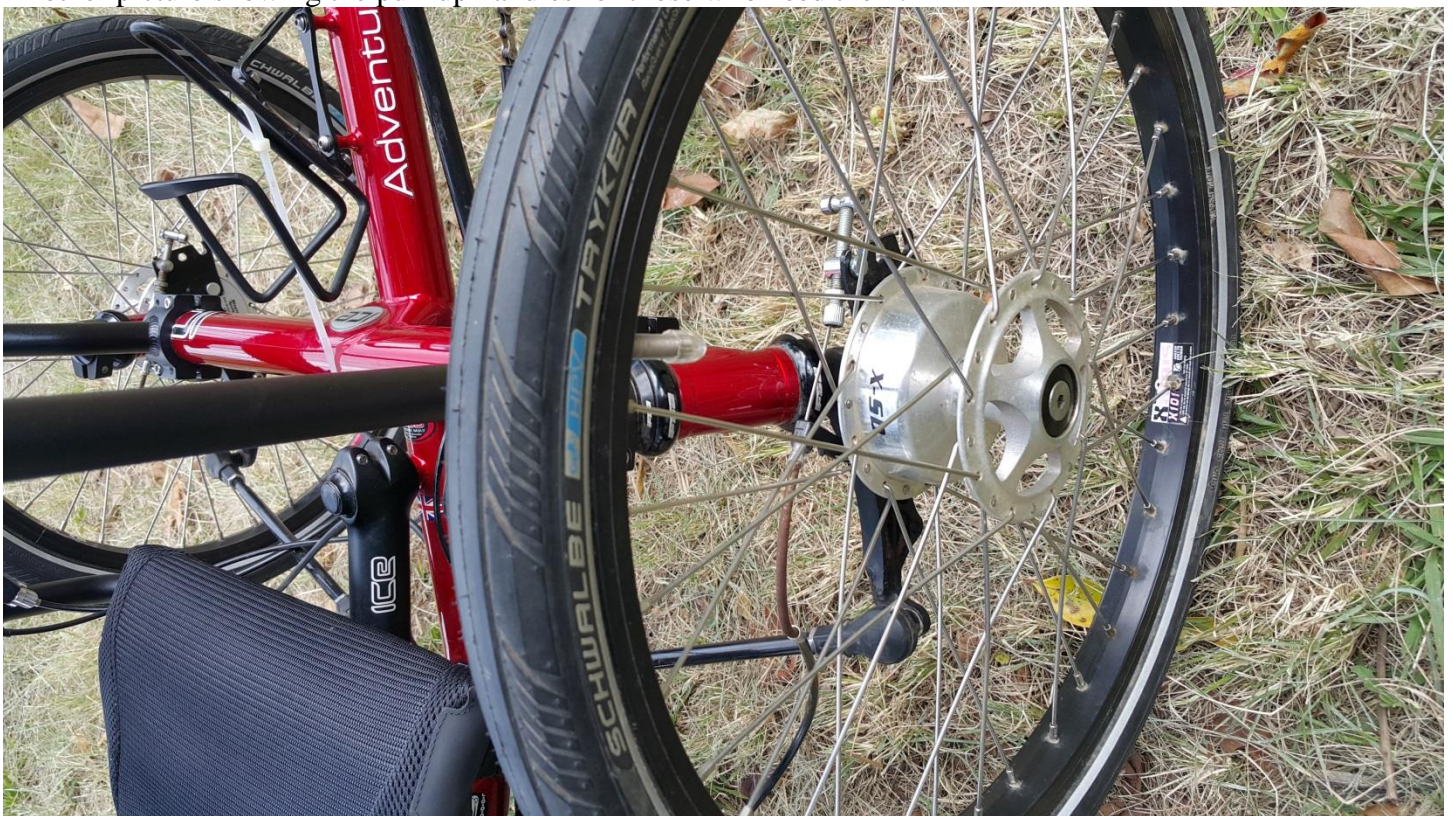
Very good quality tires and showing the drum brakes
